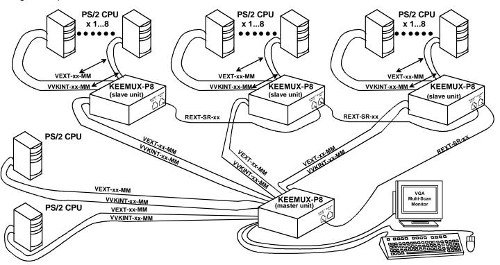
Figure 5- Cascaded configuration
